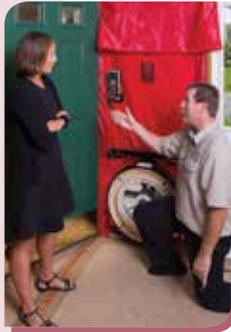
The evaluation includes a blower door test and complete insulation inspection to determine your home's insulation and air sealing potential. Uncomfortably hot rooms are often due to lack of insulation and air sealing.
